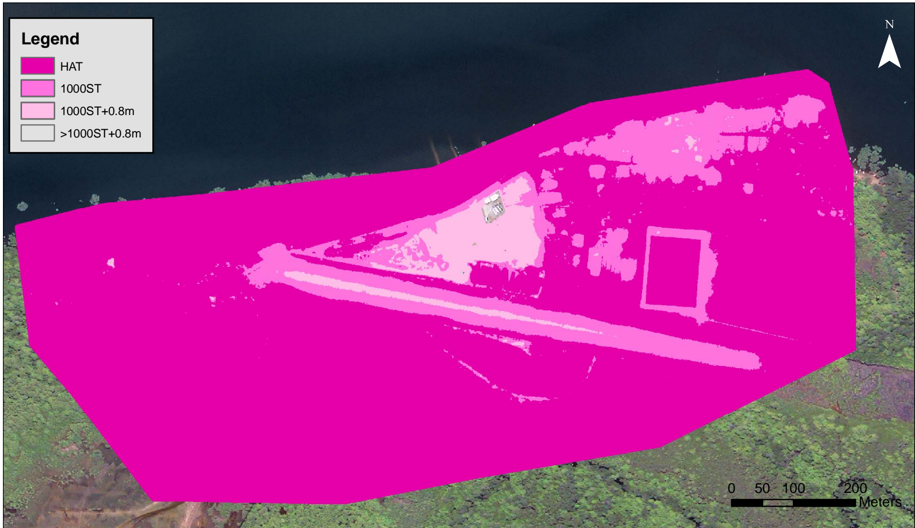
Figure 5.5c: Inundation at HAT with 1000 year return period Storm Tide and 0.8m sea level rise.
