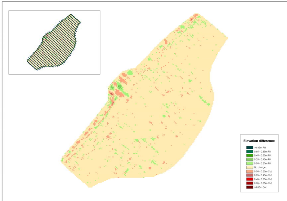
Figure 7.8: Elevation difference, 7m shore-normal dataset.
