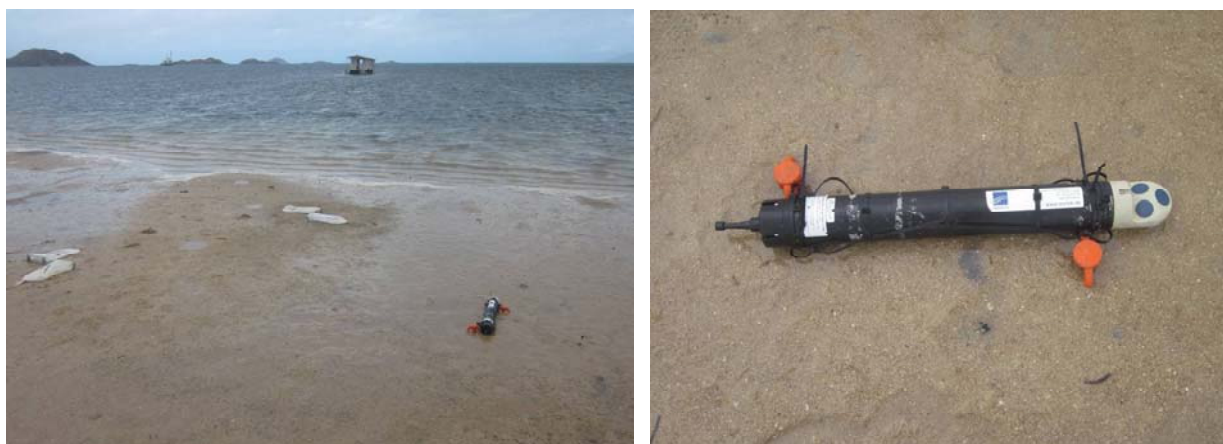
Figure 4.3: Current meter deployed adjacent to sediment traps.
