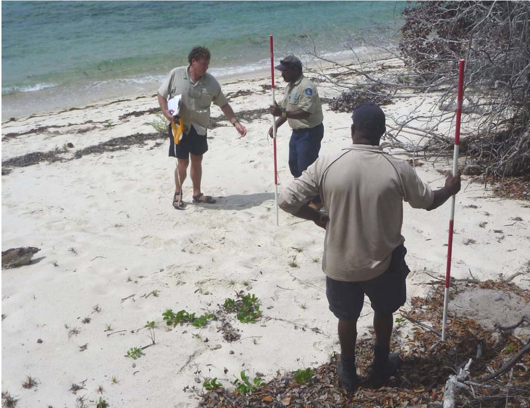
Figure 3.1: Using Emery poles to undertake a beach profile survey on Badu
